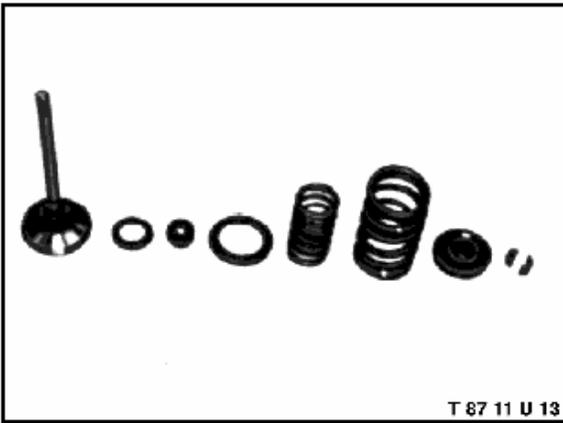
Low valve mass and dual valve springs insure reliable opening and closing between the short ignition periods.
