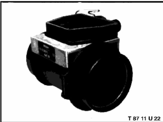
Hot wire air flow sensors are used in conjunction with Digital Motor Electronics for measurement of physical air mass. Precise and rapid load sensing allows improved adaptation to changing engine operating conditions.
