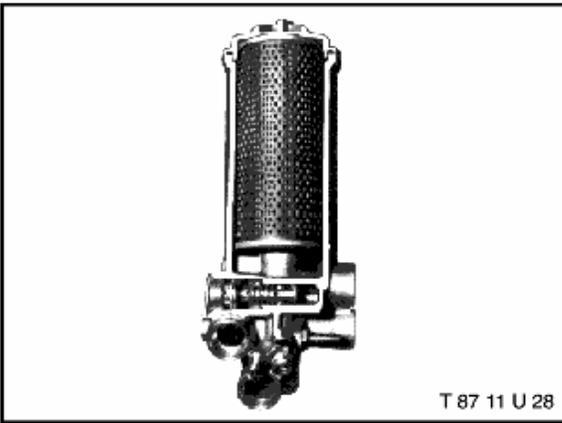
The easy access oil filter is mounted on the left inner fender. Features include large diameter hoses to insure ample oil flow and an anti-drain back valve. Thermostatic oil cooler control is located in the lower section. At a temperature threshold of 95°C, engine oil is directed to the external oil cooler for additional heat dissipation.
