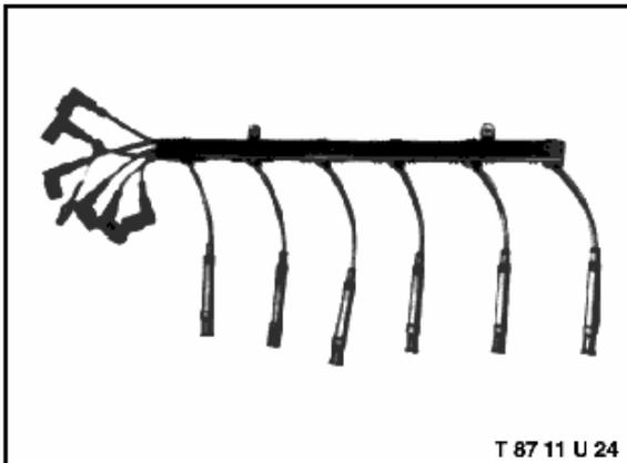
Each cylinder bank has its own secondary ignition distributor and high tension cables. All secondary wiring is routed and protected in a special plastic conduit developed for this purpose.
