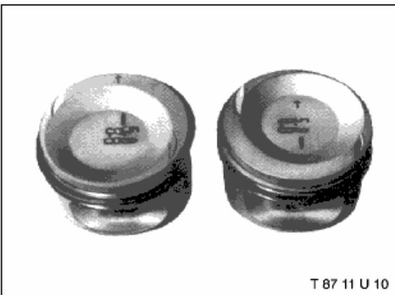
The combustion chamber bowl is located eccentrically to concentrate the air/fuel charge central to the spark plug. Correct wrist pin off-set is maintained with the use of different pistons for each cylinder bank.
