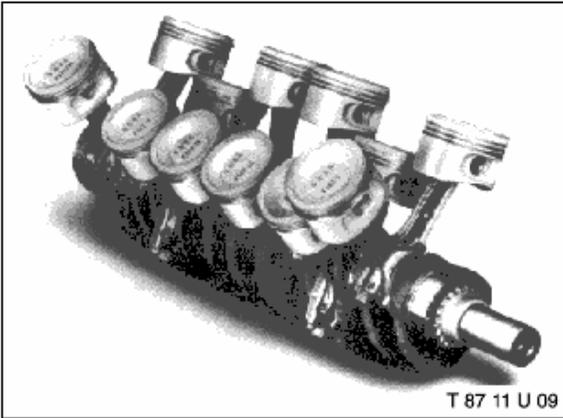
The connecting rods are made of drop forged steel and are similar to the M20 type. The center to center distance is 135mm, however, unlike the M20, the big end is machined asymmetrically. The special machining allows two rods to run on one journal, thus there is an "installed direction" requirement.
