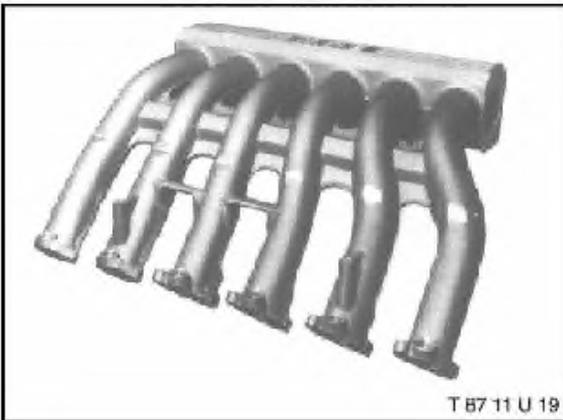
The individual cylinder banks receive precisely balanced air charge delivery from two symmetrical intake plenums which have equal length ram intake runners. The fuel injectors are mounted in the inlet flanges.
